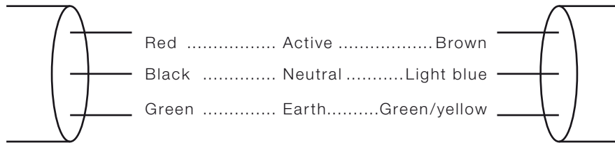
FIGURE 3.1 SINGLE-PHASE FLEXIBLE CORDS AND CABLES
